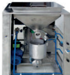
Washing Machine Central Powder Dosing System
